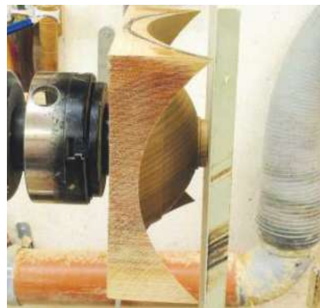
▲ Pic.15 There are a variety of designs you could choose for this bowl, such as having the bowl sat on its four corners. Due to the brittleness of the timber, I decided to sit the bowl on the central foot
